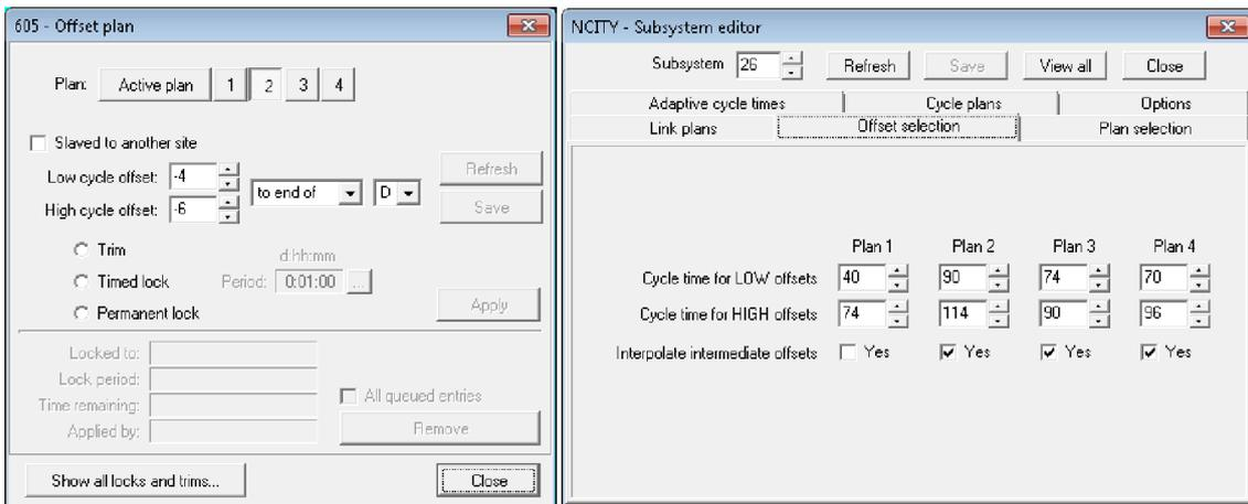
Figure 12: Offsets within a Subsystem
