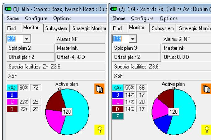
Figure 13: Active Offsets in a Subsystem
