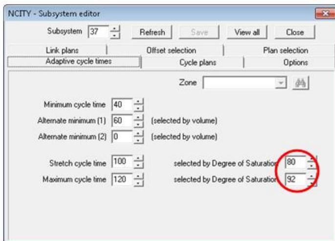
Figure 9: Subsystem sensitivity to changes in DS
